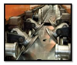
Cold-formed steel members are made from structural quality sheet steel that are formed into C-sections and other shapes usually by roll forming the steel through a series of dies. Penetrations for plumbing and electrical runs are also punched at pre-determined locations. No heat is required to form the shapes (unlike hot-rolled steel), and thus the name cold-formed steel. A variety of steel thickness is available to meet a wide range of structural and non-structural applications.
