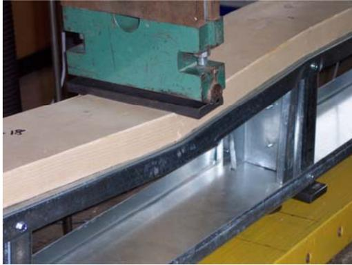
**Figure 4.9 – Deformation of Specimen 2C16-16**
