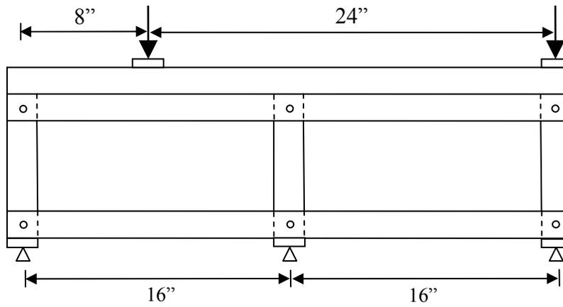
**Figure 3.1 – Typical Test Setup of 16 Inch Specimen**
