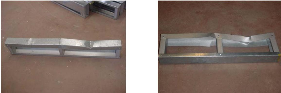
**Figure 4.16 – Bearing Failures, Specimen Group E24-18**
