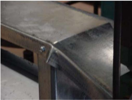
Figure 4.11-Buckling at Central Support
