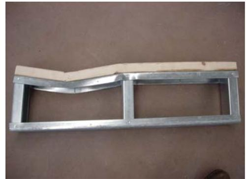
**Figure 4.2 – Flexural failure of Specimen 1A16-18**
