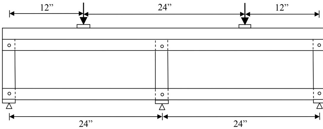
**Figure 3.2 – Typical Test Setup of 24 Inch Specimen**
