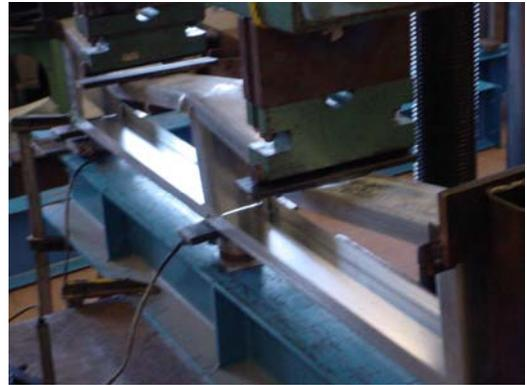
**Figure 4.8 – Failure of Specimen 2B24-16**
