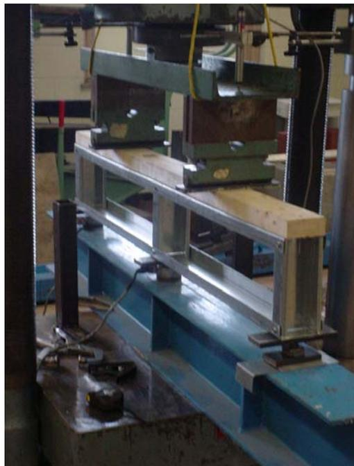
**Figure 3.3 – Typical Test Setup Showing Placement of LSCs and Load Cells**
