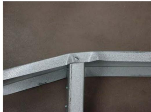
Figure 4.12-Failure of 18-ga. track
