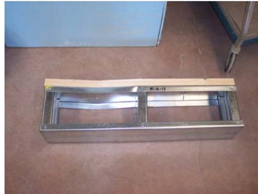
**Figure 4.10 – Preferential Span Deflection, Specimen 2C24-18**
