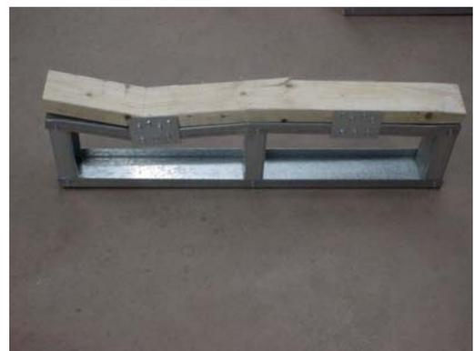
**Figure 4.4 – Note wood/track separation**
