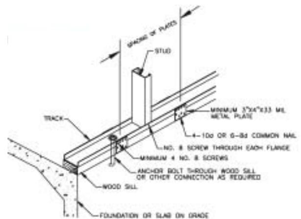
Figure E: Wall-to-Wood Sill Plate Attachment
