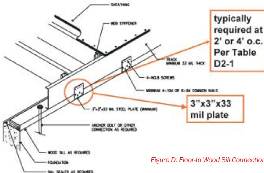
Figure D: Floor-to Wood Sill Connection
