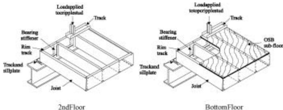
Figure 2: Sketch of test set-up and specimens
