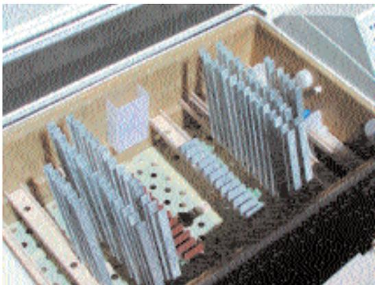
Figure 3 - Connection Specimens in Cyclic Corrosion Chamber
