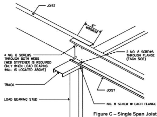
Figure C – Single Span Joist Detail
