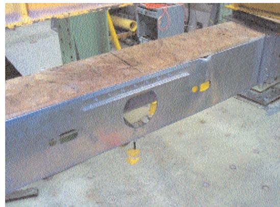
Figure 1: Hole reinforcement for flexure
