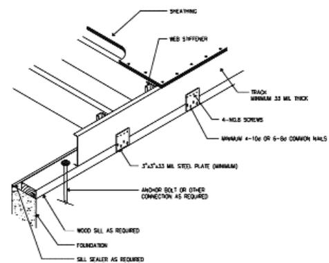
Figure D: Floor to wood sill
