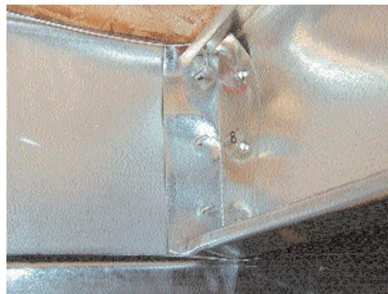
Figure 2: Web crippling of joist with 8-inch clip angle
